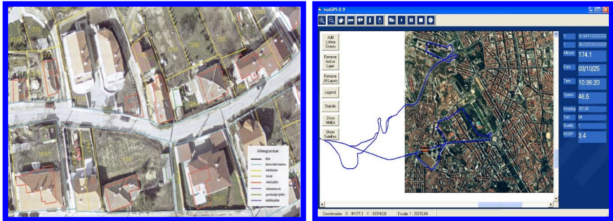
Figure 25. Examples of tool-oriented GIS applications in the smart city: on the left, a building survey showing the real (aerial photo) and land registry (red line) locations of residential properties (such applications can be used for building fines, as they provide evidence of unauthorised construction). On the right, a tool-oriented GIS application for public transport combined with GPS.
