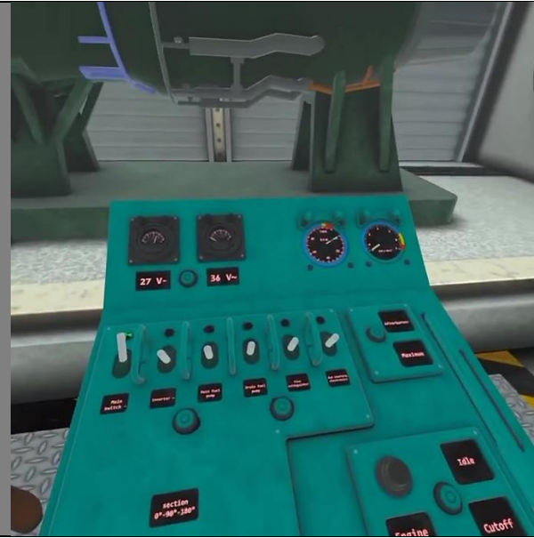
Figure 4. Real-time Status Monitoring and Instrument Feedback. Close-up view of the instrument clusters and status indicators. Voltage readings and circuit adjustments form a synchronous feedback system, enabling the user to interpret measurement data and comprehend the causal relationships between parameter changes and system behaviour.
