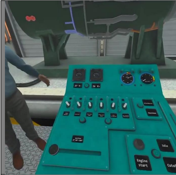
Figure 3. Overview of the Interactive Control Console. The primary interface for system interaction, featuring levers, switches, and analogue gauges. This hybrid UI solution replicates authentic industrial logic while facilitating the acquisition of operational sequences through integrated feedback and intervention points.
